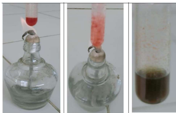
Figure 2. Testing for the presence of anthocyanins in the extract was conducted via color reactions using hydrochloric acid and sodium hydroxide reagents.
