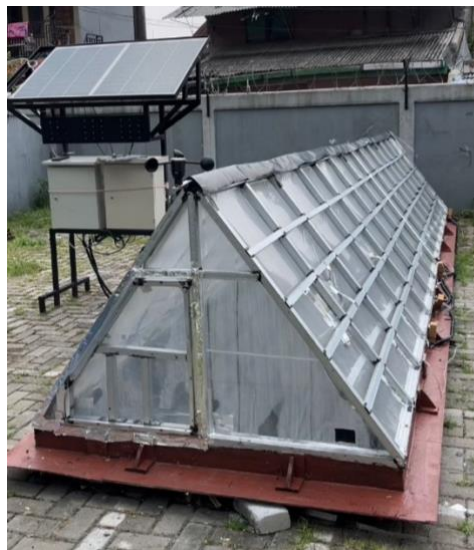
Figure 3. Solar still desalination process
