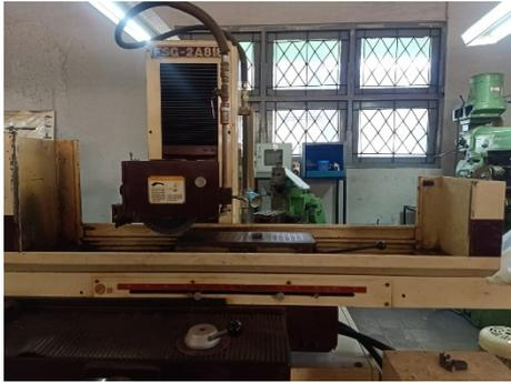
Gambar 10. Proses grinding
