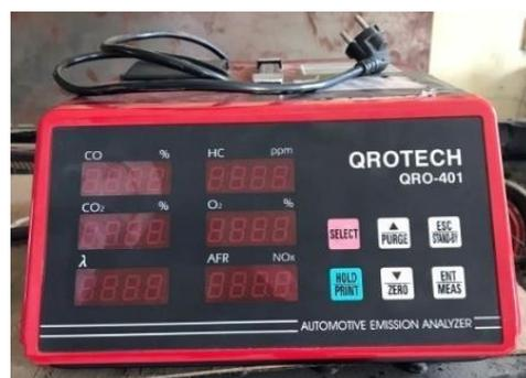
Gambar 1. Gas Analyzer QROTECH - 401
