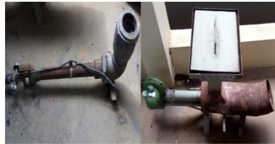
Gambar 6. Burner (a) Burner gas; (b) Burner RDF
