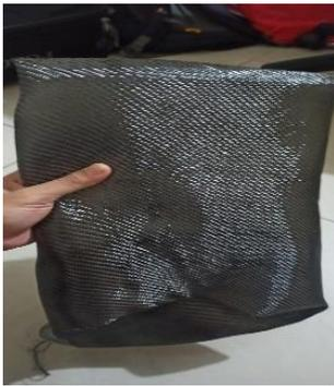
Gambar 3. Serat karbon 3K 220 gsm model Twill
