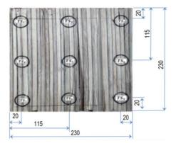
Figure 11. Position of eight measurement points on specimen 1 (unit of measure in mm)
