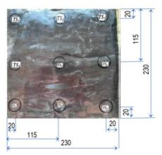
Figure 12. Position of eight measurement points on specimen 2 (unit of measure in mm)
