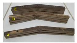
Figure 19. Condition of specimen after test; (a) 3 layer; (b) 4 layer; (c) 5 layer
