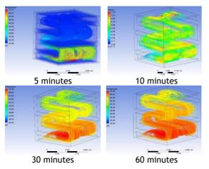
Figure 17. Result of analysis of temperature distribution for 60 minutes
