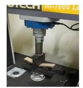
Figure 18. Bending test on 5-layer bamboo lamination specimen
