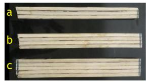
Figure 9. Bending test specimen; (a) 3 layers; (b) 4 layers; (c) 5 layers
