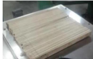
Figure 2. Specimen 1 (bamboo lamination)
