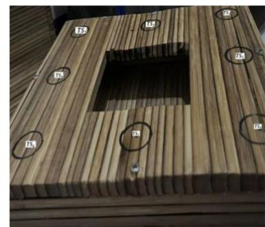
Figure 15. Position of temperature measurement point
