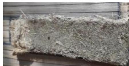
Figure 6. Combination of lamination and bamboo fibers
