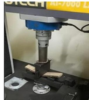
Figure 18. Bending test on 5-layer bamboo lamination specimen
