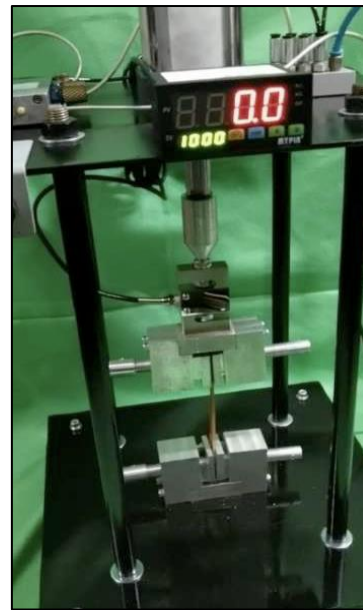
Figure 1. Tensile test machine up to 2 kN capacity (Zariatin, Kurniawan and Ikhsan, 2021)
