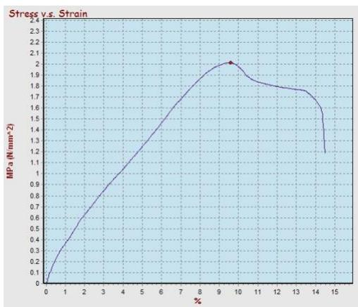
Figure 16. Tensile strength graph of sample KR50KS50
