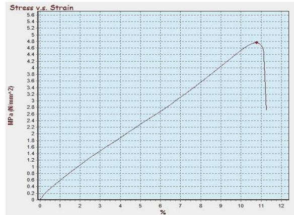
**Figure 13.** Tensile strength graph of sample KR60KS40
