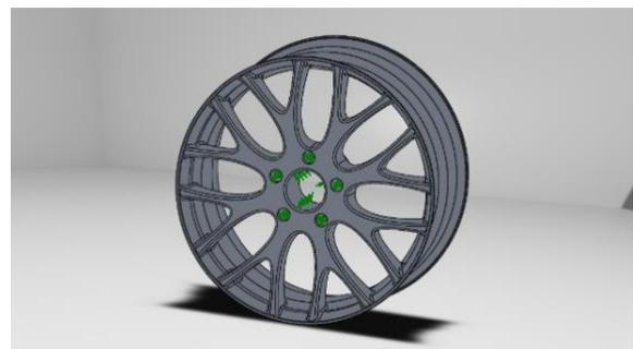
Figure 6. Fixed geometry load point.
