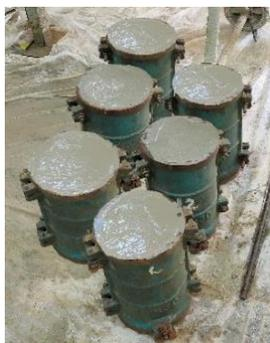
Figure 4. Concrete cylinder
