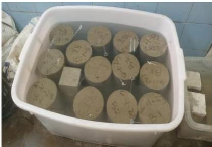
Figure 7. Concrete immersing with seawater.
