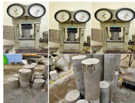
Figure 9. Concrete cylinder loading.
