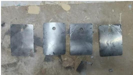
Figure 4. SPSS specimen after being sanded random orbital sender.
