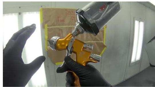
Figure 3. Feed spray gun (Devilbiss GTI Pro Lite Gravity).
