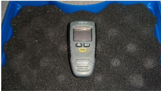
Figure 11. Coating thickness gauge.
