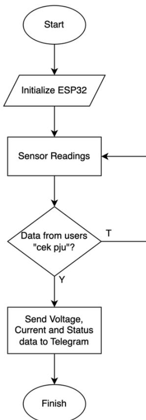
Figure 5. PJU checking flowchart.
