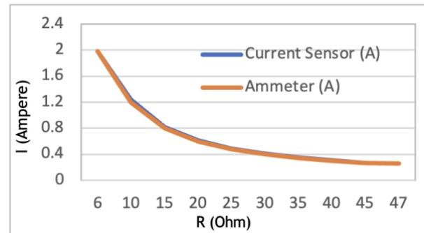
Figure 9. Chart current sensor comparison with an ammeter.
