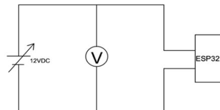
Figure 10. Suite voltage sensor test.
