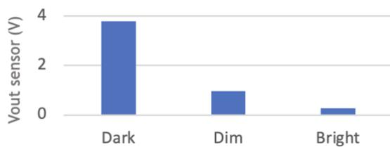
Figure 12. Chart results LDR sensor testing.
