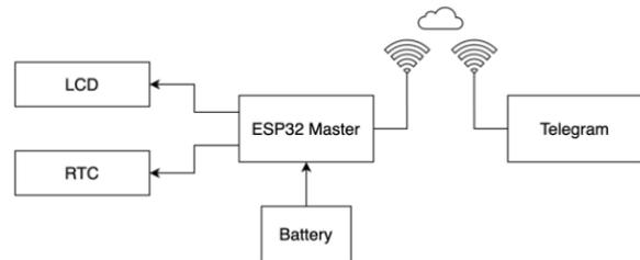
Figure 3. Master block diagram.
