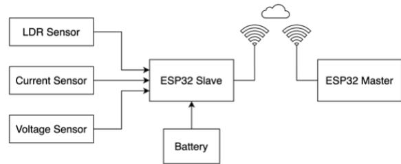
Figure 2. Slave block diagram.
