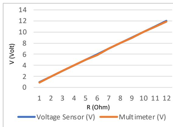
Figure 11. Chart voltage sensor comparison with multimeter.
