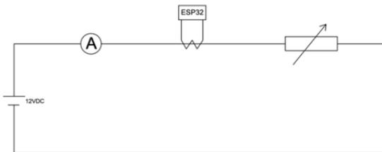
Figure 8. Suite ACS712 current sensor testing.
