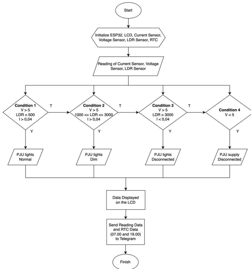
Figure 6. Flow diagram of sending telegram message notifications to users.
