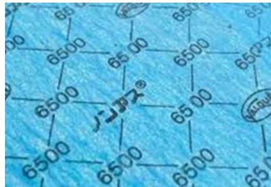
Figure 14. Gaskets used in the FSSW process.
