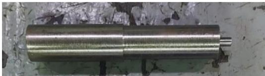
Figure 3. Tool shoulder with 7 mm pin (after turning).
