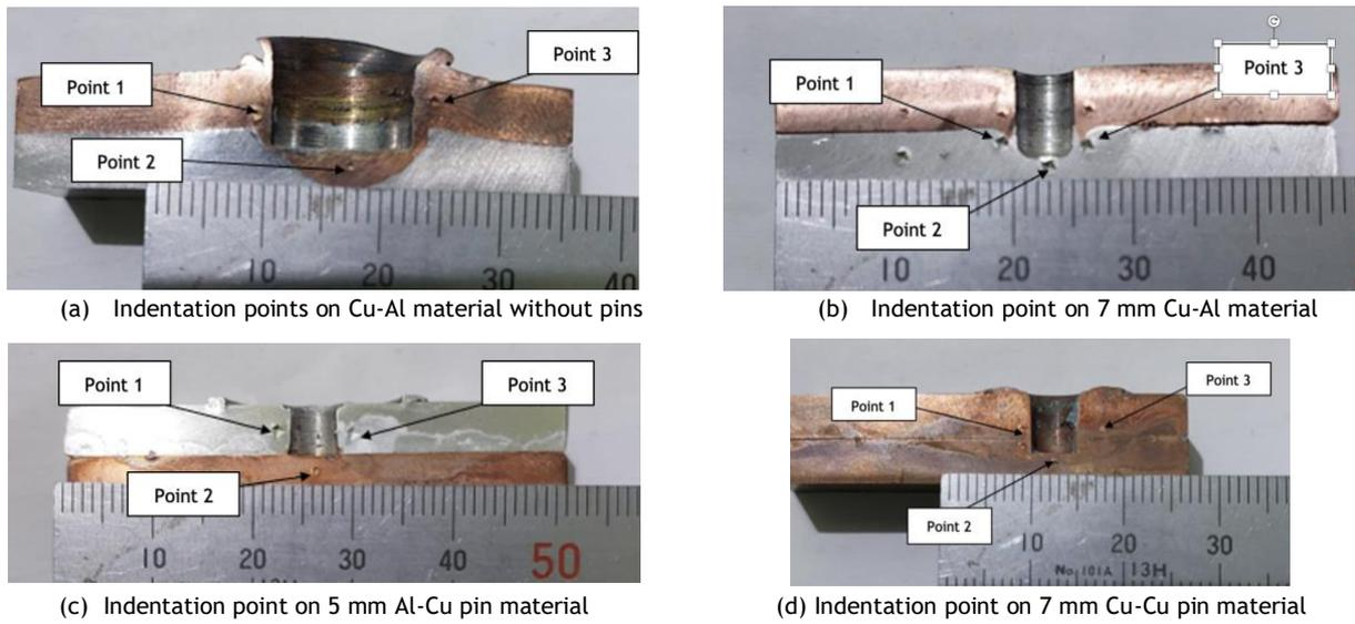
Figure 25. Indentation points of samples.
