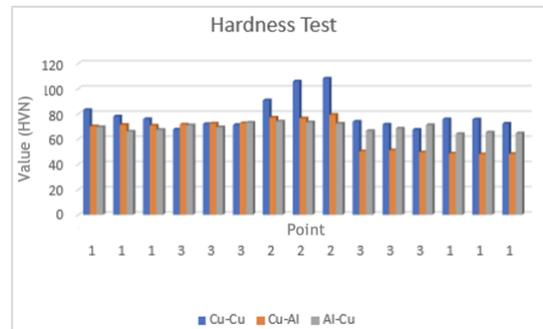
Figure 26. Histogram of hardness test.
