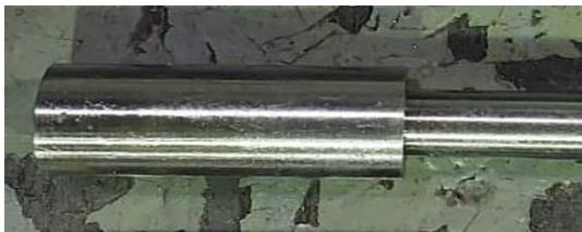
Figure 5. Tool shoulder without pin (after turning).
