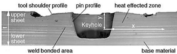
Figure 17. Microphoto position of the test sample (Bilici, 2012).
