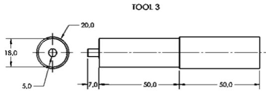
Figure 11. Shoulder with pin size 7 mm x 5 mm.
