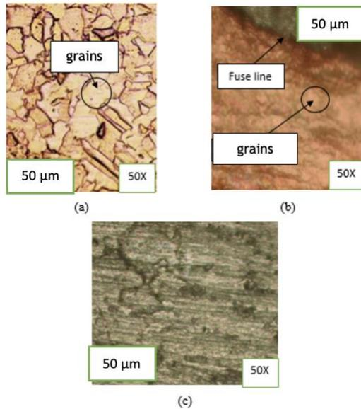
Figure 23. Microstructure of HAZ (a) Cu-Cu, (b) Cu-Al and (c) Al-Al.
