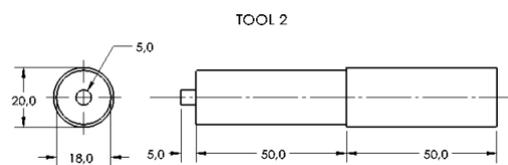
Figure 10. Shoulder with 5 mm x 5 mm pin.
