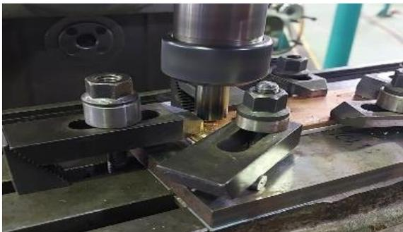
Figure 12. Clamping Kit used in the FSSW process.
