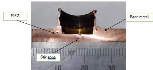
Figure 21. Position for a micro photo of the test sample.
