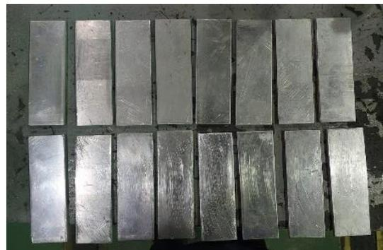
Figure 8. Aluminum material 150x50x5 mm.
