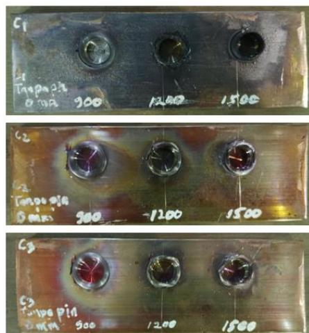
Figure 20. Samples C1, C2, and C3 top view of FSSW welding without pin (0 mm) welding depth of 2 mm.
