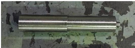
Figure 4. Tool shoulder with 5 mm pin (after turning).
