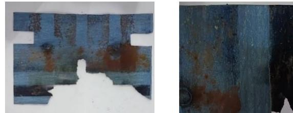
Figure 15. Condition of the gasket after being used in the FSSW process.
