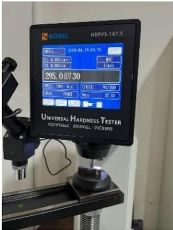
Figure 16. Hardness testing.
