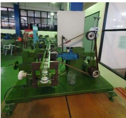
**Figure 5.** Centerless belt grinding machine.
