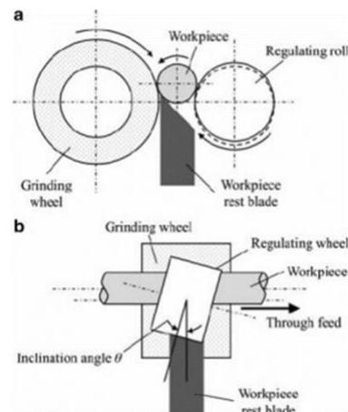
Figure 10. Centerless belt grinding parameters (Leonesio, Bianchi and Safarzadeh, 2019).
