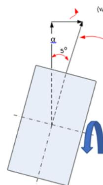
Figure 11. Illustration of the influence of adjustment wheel tilt on the amount of feeding speed  $V$ .
