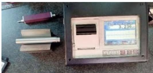
Figure 9. Roughness tester.
