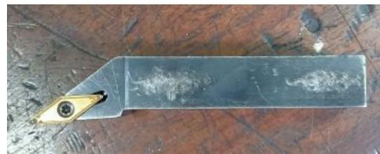
Figure 2. Chisel lathe VBMT 160408HQ.
