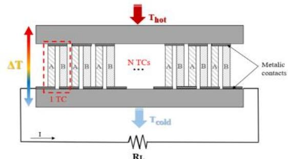
Figure 8. Temperature system TEG.
