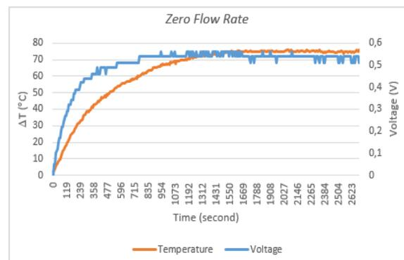
Figure 10. Voltage output TEG at zero flow rate.
