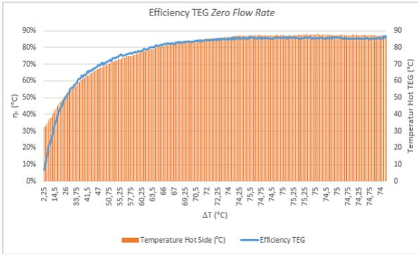
Figure 12. Efficiency of TEG at zero flow rate.
