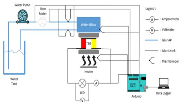
Figure 7. Design of TEG testing equipment.
