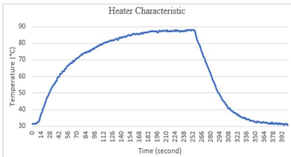
Figure 9. Heater characteristic.
