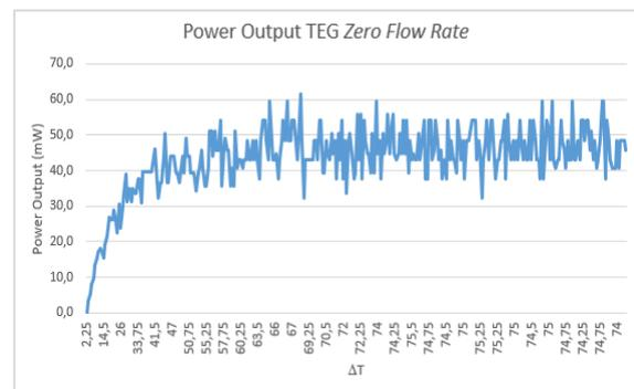
Figure 11. Power characteristics at zero flow rate.
