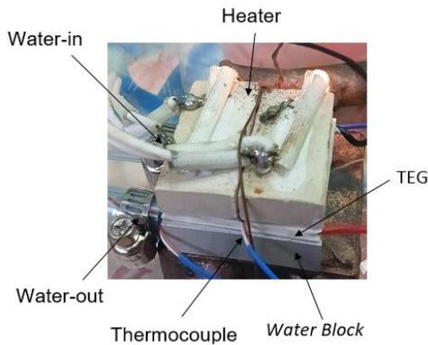
Figure 6. Water block position and the series
