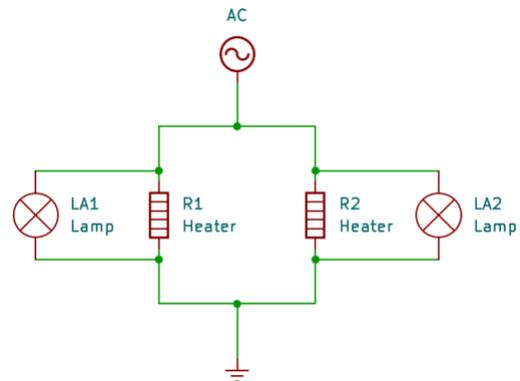
Figure 3. Wiring diagram heater.
