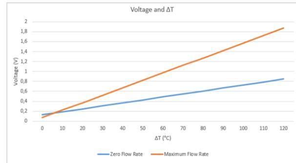
**Figure 18.** Output voltage TEG SP1848 27145 SA.
