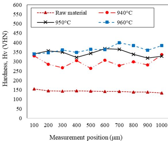
Figure 10. Internal hardness of the jaw implant at the inner radius.
