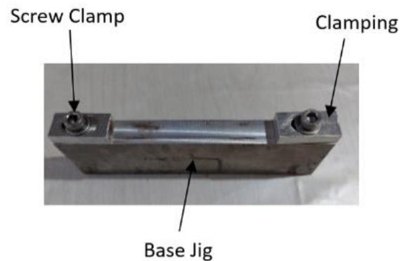
Figure 2. Jig used to hold the workpiece in the EDM process.
