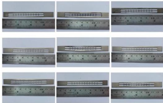
Figure 4. Jaw implants produced by the die-sinking EDM process.
