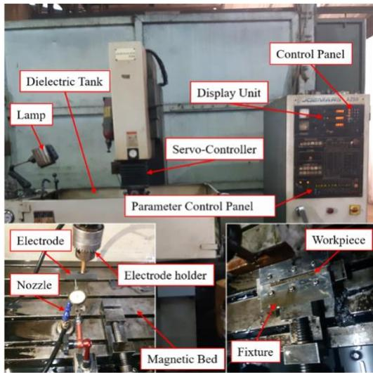
Figure 3. CNC EDM Die-sinking Machine (JOEMARS AZ50) (Kurniawan *et al.*, 2023).
