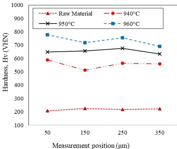
Figure 8. Hardness of the WL on the outer radius of the jaw implant.
