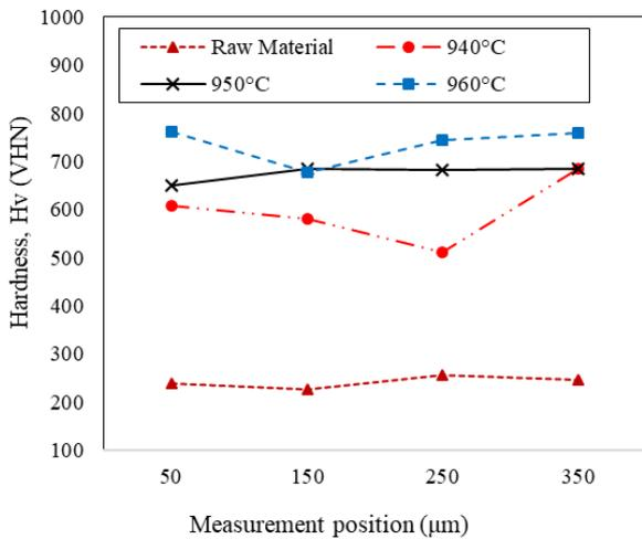
Figure 7. Hardness of the WL on the inner radius of the jaw implant.
