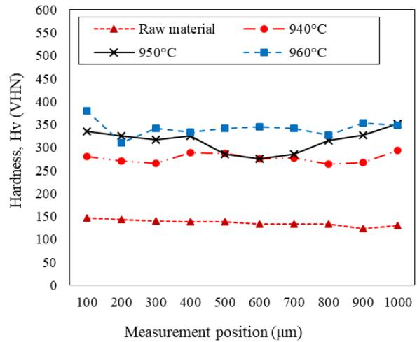
Figure 11. Internal hardness of the jaw implant at the outer radius.
