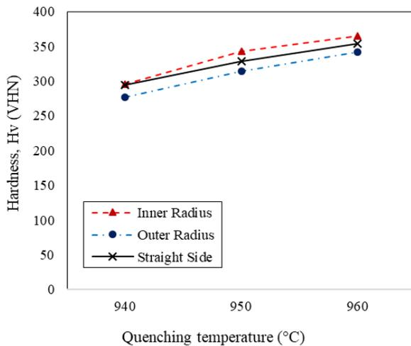
Figure 13. Relationship between quenching temperature and jaw implant hardness.
