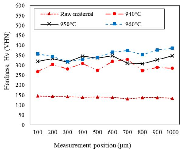
Figure 12. Internal hardness of the jaw implant on the straight side.
