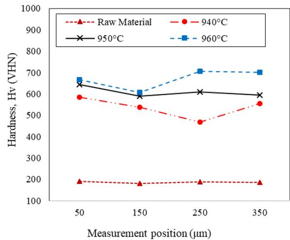
Figure 9. WL hardness on the straight side of the jaw implant.
