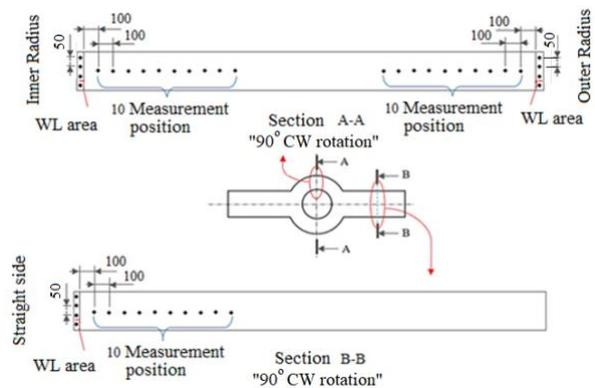
Figure 6. Position of jaw implant hardness measurement.
