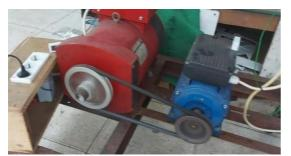
Figure 1. Generator and motor set.
