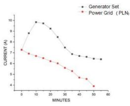
Figure 6. Rectifier current graph when charging battery with two sources.
