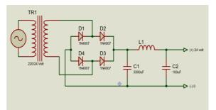
Figure 3. Circuit of a converter (Agarwal, 2023).
