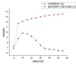
Figure 8. Battery charging: battery current and voltage graph with generation source.
