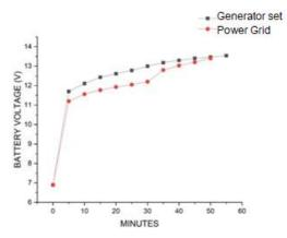
Figure 7. Rectifier voltage graph when charging battery with two sources.
