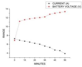
Figure 9. Battery charging: battery current and voltage graph with power grid (PLN).
