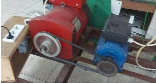
Figure 1. Generator and motor set.
