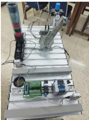
Figure 2. MPS distribution station ( FESTO, 2007 ).
