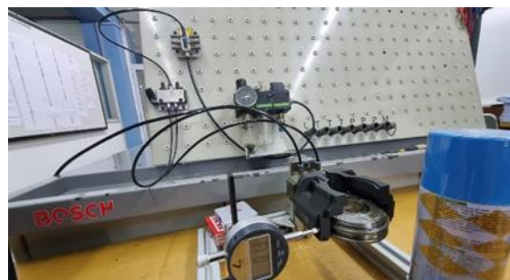
Figure 8. Deflection testing of jaw gripper.
