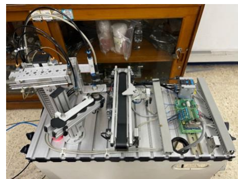
Figure 2. Pick and place station (Siva, Irawan and Utama, 2023).
