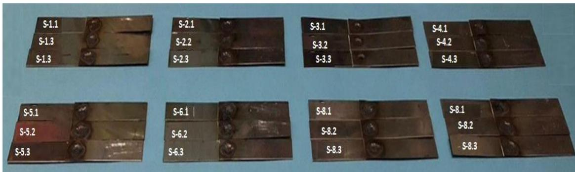
Figure 3. TIG-welding coupon: 24-unit sample from 8 iterations of SUS 304 steel sheets.
