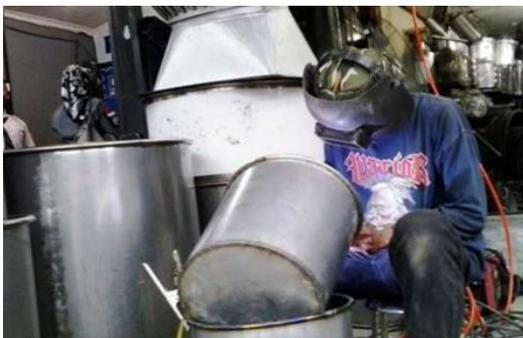
Figure 1. TIG-welding application on pan handles (Media, 2018).
