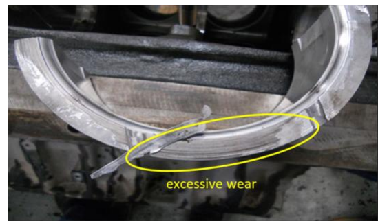
Figure 4. Rear shaft wear.
