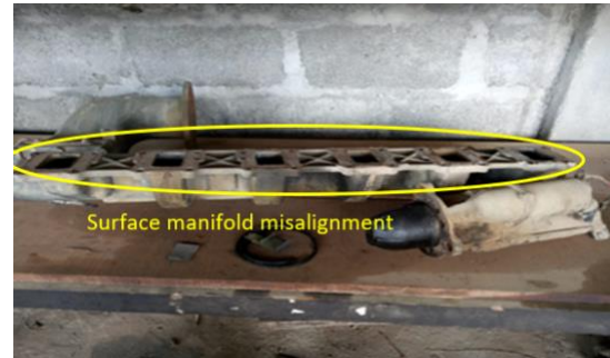
Figure 6. Exhaust manifold trouble.
