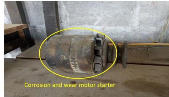
Figure 5. Motor starter trouble.
