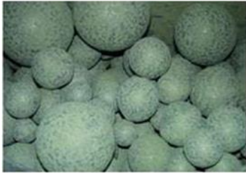
Figure 9. The surface of steel balls in the ball mill without CGA (Kalkan, 2023).
