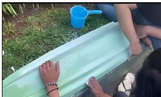
Figure 8. External hull coating with putty
