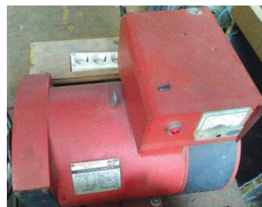
(b). Synchronous AC Generator 1 phase
