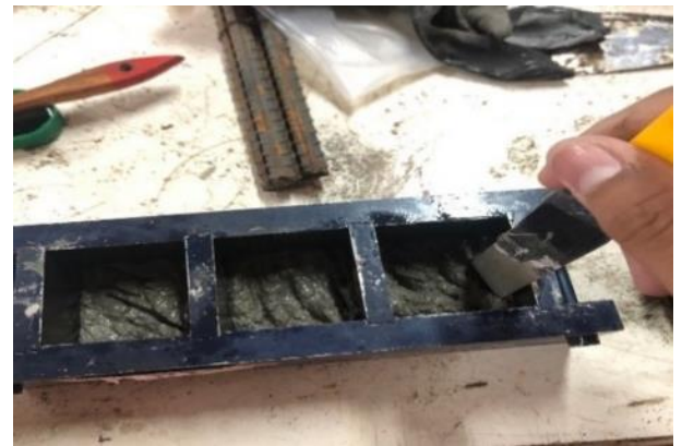
Figure 2. Making of test specimens
