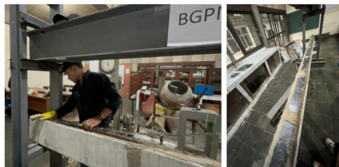
Figure 11. Installation process of CFRP sheets on the beam specimen
