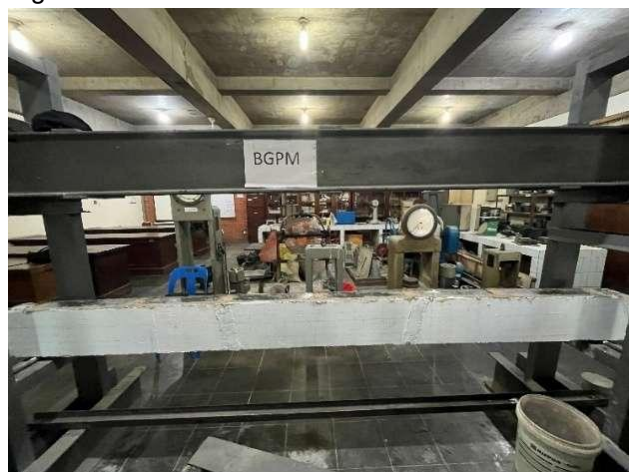
Figure 12. The beam specimen after repaired and strengthened
