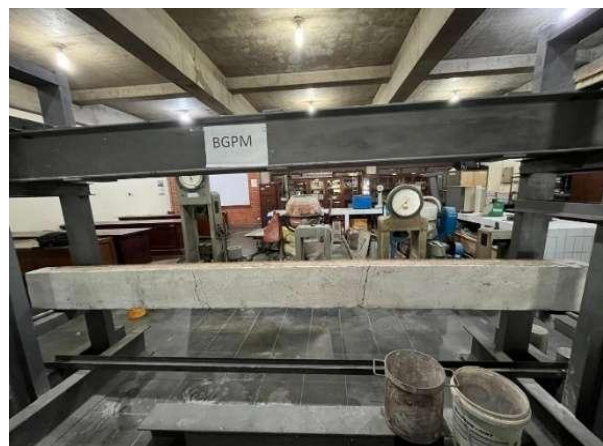
Figure 1. Longitudinal view of the beam specimen before repair and strengthening
