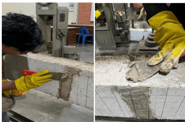
Figure 10. Application of Sikadur-31 CF epoxy to the cracked zone
