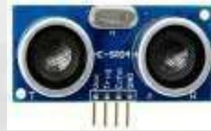
Gambar 7. Sensor Ultrasonik HCSR 04
