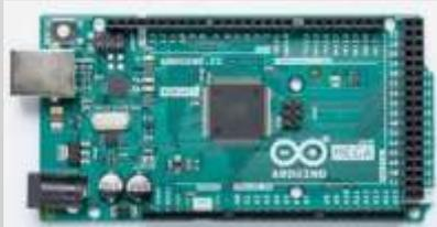
Gambar 4. Arduino Mega
