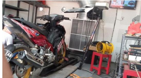
Gambar 2. *Computerised Chasis Dynojet*
