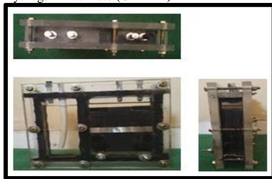
Gambar 4. Foto Generator Elektrolizer Hydrogen Zinc Plate (GEH-ZP)
