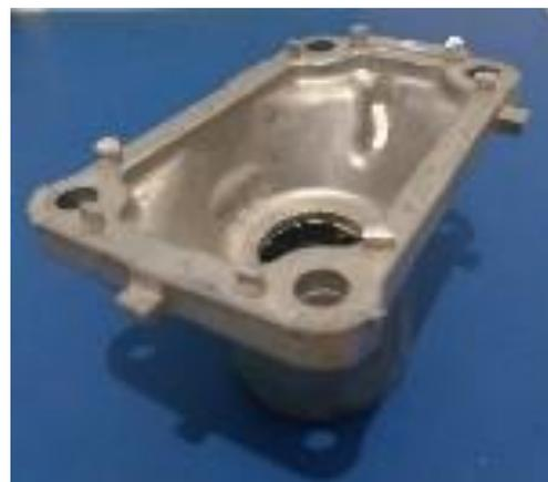
Gambar 2. Retainer Control Shift Lever
