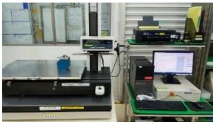
Gambar 18. Mesin *Surface Test* (*Roughness Tester*)
