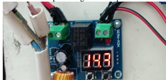
Gambar 12. Modul Low Voltage Disconnect Protection Battery
