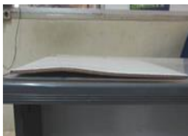
Gambar 10 Defect Weavy Surface
