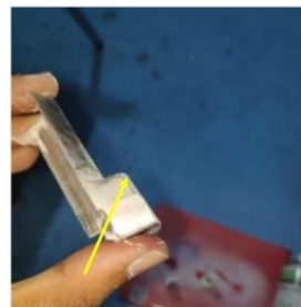
Gambar 12 Blade Rotor Nonrelevant Indication
