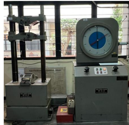
Gambar 4. Proses uji tarik specimen
