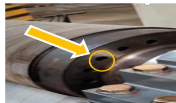
Gambar 3 Lubang vacuum flutting corrugator BHS
