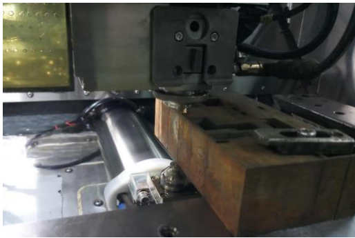
Gambar 8 Proses WEDM Chuck TFV
