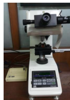
Gambar 7. Alat uji kekerasan Vickers Microhardness Tester FM-310.
