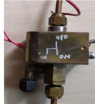
Gambar 4 *Koil Solenoid Valve*
