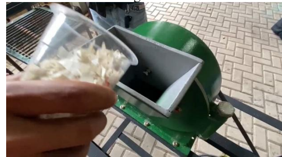
Figure 4. Testing Machine With HDPE Plastic
