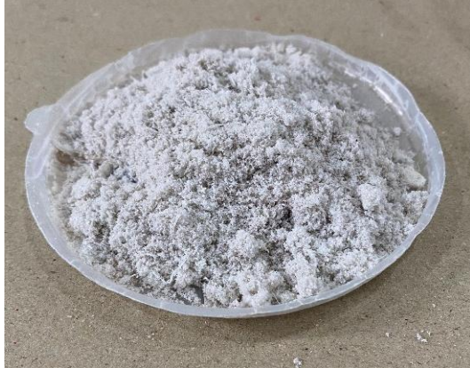
Figure 6. HDPE Plastic Fine Powder After Finishing
