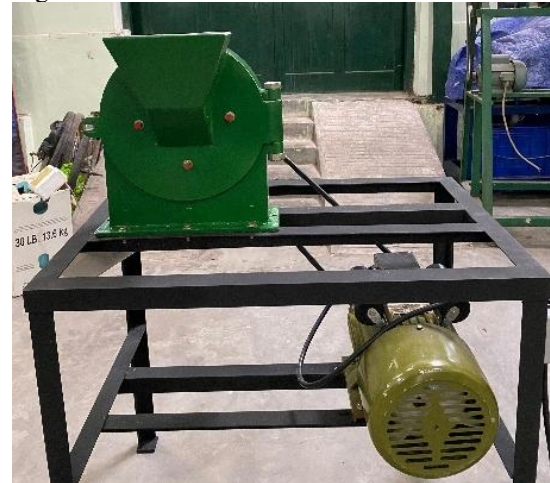
Figure 3. HDPE Plastic-Free Machine Testing Next is testing using HDPE plastic. This test is carried out to find out if the machine can function optimally and produce the expected output. This test is carried out twice with a time difference applied. The testing of HDPE plastic crusher machine is shown in Figure 4.
