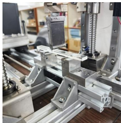
Figure 14 Bending test on the designed testing machine
