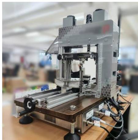
Figure 9 Results of the designed bending test machine construction
