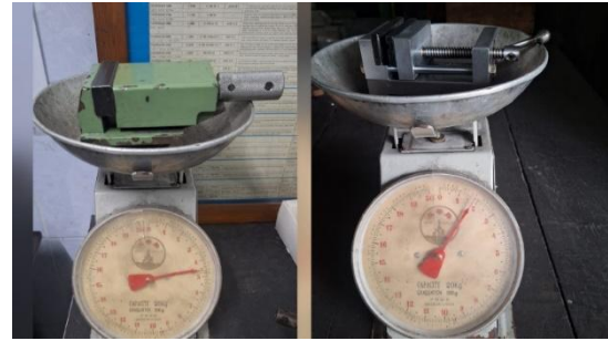
Figure 6. The original vice weigh in (left) and the redesigned vice weigh in (right).
