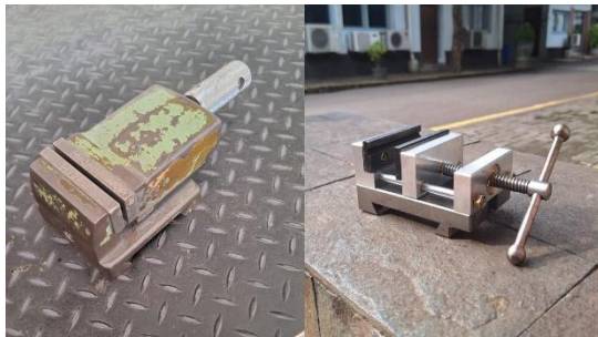
Figure 5. Actual physical comparison between the original vice (left) and the redesigned vice (right).
