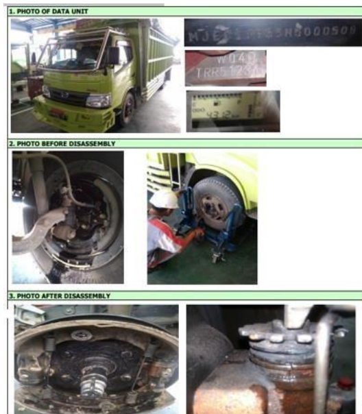
Figure 1. One example of a truck that has a brake oil leak
